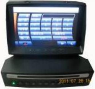
A black digital car stereo unit with a small screen displaying a menu. Below it is a black base unit with a digital display showing "2011-07-26 15".                                           | Landrover Discovery 3  | <ul style="list-style-type: none"> <li>* 7" Digital 800*RGB*480 touch screen</li> <li>* Bluetooth/AM/FM/TV/Amplifier</li> <li>* Ipod control/USB/SD ready</li> <li>* Steering wheel control</li> <li>* GPS build-in</li> </ul> |  |
